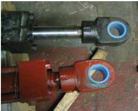
ThorPlas-Blue steering and linkage bearings installed
