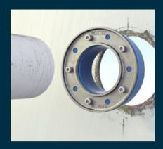
Slide the pipe through the Roxtec SPM seal and insert it into the opening. The seal copes with wide tolerances towards both pipe and opening.
