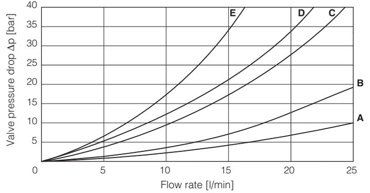
**17 OPERATING LIMITS** based on mineral oil ISO VG 46 at 50°C
