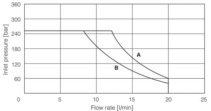
**18 INTERNAL LEAKAGES** based on mineral oil at viscosity 15 cSt
