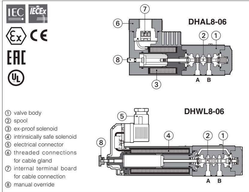
On-off directional valves size 06 in **low leakage execution**, equipped with **Ex certified solenoids**, ideal for hydraulic systems assisted by accumulators operating in hazardous environments.
