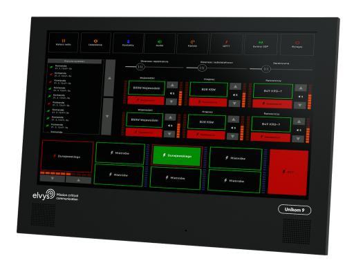
The console allows the connection of external devices such as headphones or headsets, external microphone with PTT button and PTT footswitch, telephone handset, keyboard, mouse, etc.
