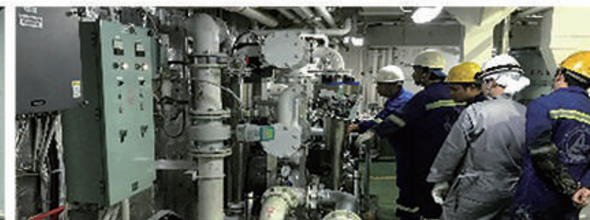
Ship Owner □ Japa (Toko Kaiun)L | Ship Type □ Tanker Pump Capacity □ 150m 3 / h x 1 | Model □ BSKY 150 x 1 set Skid Type Class □ CCS / LR
