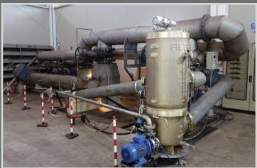
Filter ACB-9100 on test bench: Flowrates up to 4.200 m<sup>3</sup>/h
