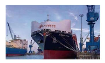
• The wind resistance of ships accounts for more • Therefore, the research on wind resistance reduction with a large wind-affected area of the superstructure is gradually attracting attention.
