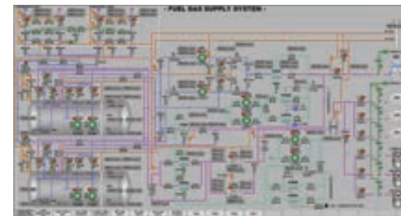
Control MIMIC for Fuel Gas Supply System
