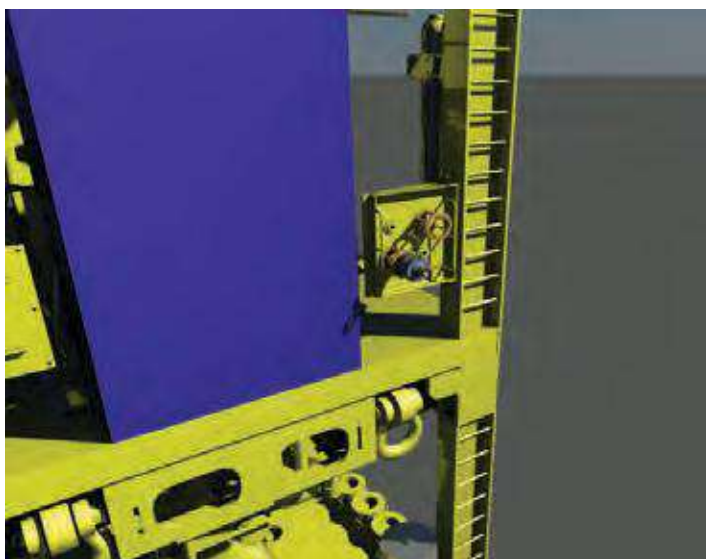
LMRP ROV wireless data and power connection point and ROV retrievable black box recorder
